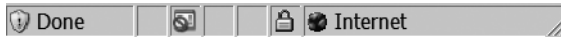
Figure 11-14. The lock icon in the browser shows that the current web session is encrypted.
